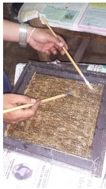
Figure 3. Mixing Epoxy Resin and Hardener with Ramie fiber Reinforcement in to the Mold
