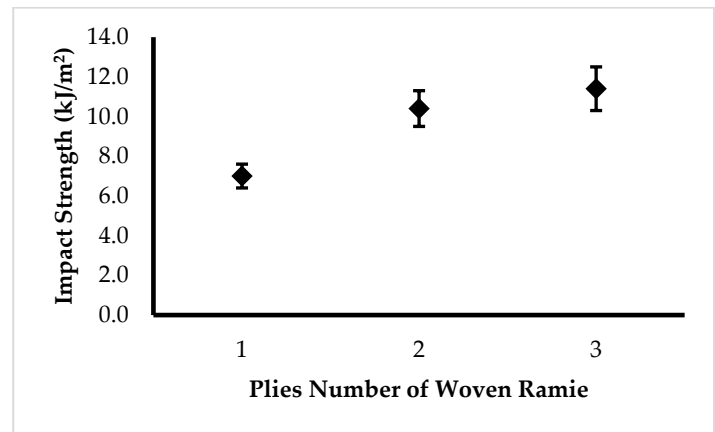
Figure 5. The Relations Between the Plies Number of Woven Ramie Composite to the Impact Strength
